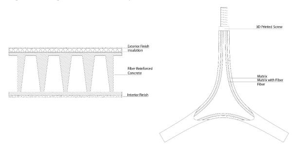
Figures 1 and 2: Detail of material distribution in a wall horizontal section
