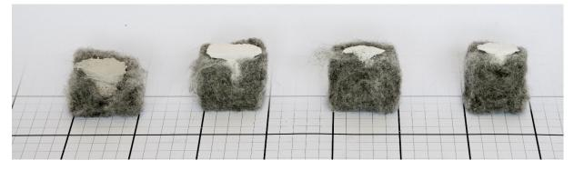
Figure 3: Sections of specimens of felted fiber. From left to right 0.032g/cm3, 0.064g/cm3, 0.096g/cm3 and 0.128g/cm3. All of them infused with the same amount of plaster
