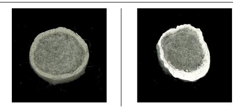
To calibrate the density of needle felted material for the matrix infusion process, a series of differently dense specimens were tested, as shown in Figure 3:
