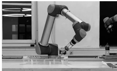
Figure 12 Robotic injection process within suspension
